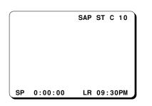
O To remove the status display, press the DISPLAY button (press the button twice if a tape is loaded in the VCR).
